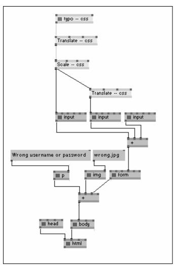
Fig. 6: A HTML tree with allocated CSS nodes
