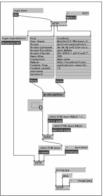
Fig. 4: The login verification graph.
